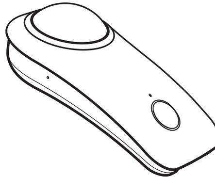
Recording is stopped by manually short pressing the Sr600 main power/record button or via an input that has been configured to stop recording.
